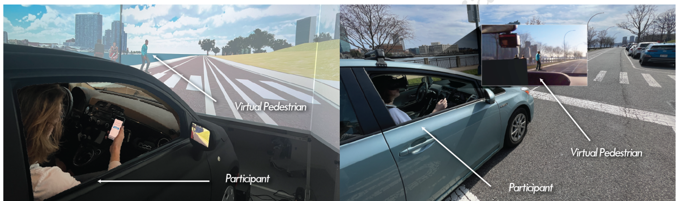
Figure 1: Portobello enables platform portability , so that the same study can be run on in-lab (left) and on-road (right) driving simulation platforms.
